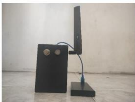
Fig. 6 LoRa Node (left) and LoRa Gateway (right)
